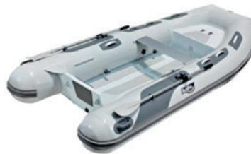
We manufacture and sell the *Poseidon HB-310AX* rigid inflatable boat (RIB)\*<sup>5</sup>, which adopts aluminum material for the boat bottom to facilitate recycling at the time of disposal.
