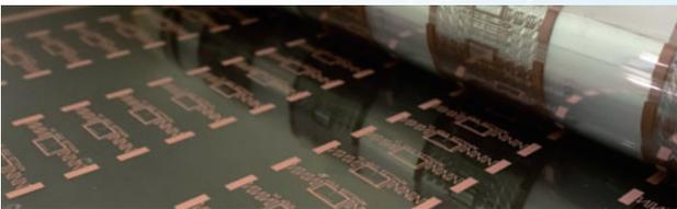
Polypyrrole plating is an electroless plating technology commercialized as a result of development spanning more than ten years, starting in 2003. This is a technology created from the project STEP, which is an acronym for Surface finish Technology for Electroless Plating, named in-house. Polypyrrole plating has a lower environmental impact than conventional plating processes, contributes to energy-saving, and enables development of applications in a wide range of areas.
