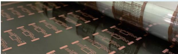
Polypyrrole plating is an electroless plating technology commercialized as a result of development spanning more than ten years, starting in 2003. This is a technology created from the project STEP, which is an acronym for Surface finish Technology for Electroless Plating, named in-house. Polypyrrole plating has a lower environmental impact than conventional plating processes, contributes to energy-saving, and enables development of applications in a wide range of areas.
