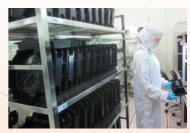
Wafer shipping cases being thoroughly cleaned in Achilles' clean room facility
