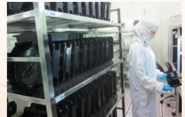
Wafer shipping cases being thoroughly cleaned in Achilles' clean room facility
