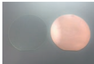
Appearance of glass substrate before plating (left) → after plating (right)
