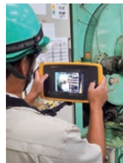
Scene from worksite inspecting air leak locations using an ultrasonic camera
